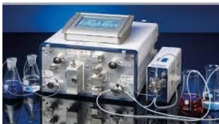
H-Cube Pro (ThalesNano) (In-flow hydrogenation)
